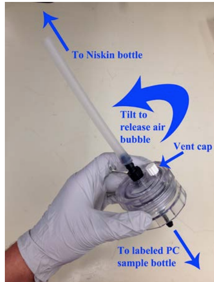
Figure 14. Capped inline filter holder with GF/F filter inserted underneath O-ring. Connect silicone tubing to Niskin bottle, begin the flow of sample and tilt so air bubble is underneath vent cap. Carefully loosen vent cap to release air bubble, tighten, and then begin rinsing labeled PC bottle with filtrate three times before filling to ~50 mL mark. Bottles can be carried to Niskin bottle rosette using the provided sampling tray (Fig. 15).
