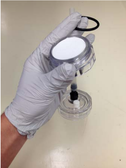
Figure 12. Inline filter holder with O-ring removed and GF/F filter inserted.
