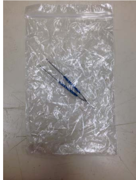
Figure 6. Forceps. Should be rinsed (Fig. 7) after removing used filter (i.e., after every station collection).
