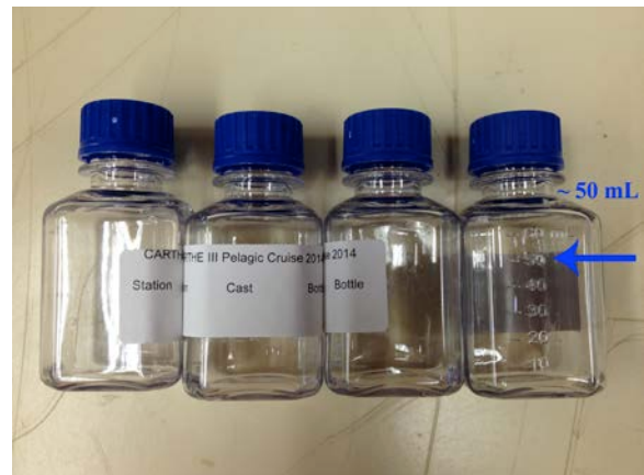
Figure 4. Pre-labeled PC sample bottles. Sampler will need to include station, cast and bottles numbers.
