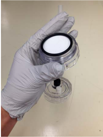
Figure 13. Inline filter holder with O-ring placed on top of inserted GF/F filter.
