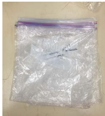
Figure 16. Ziploc® bags for storing frozen samples. Each bag can fit twenty-four 60 mL PC bottles.
